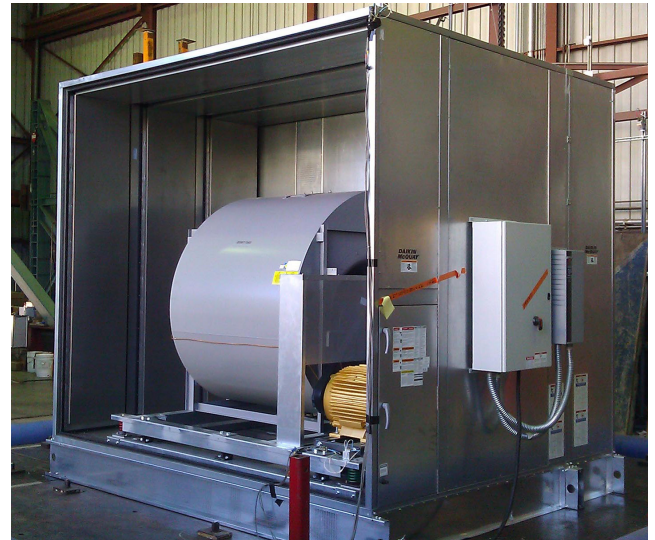
Daikin Vision® air handler OSHPD pre-approval seismic testing on the University of California, Berkeley Pacific Earthquake Engineering Research (PEER) shake table.
